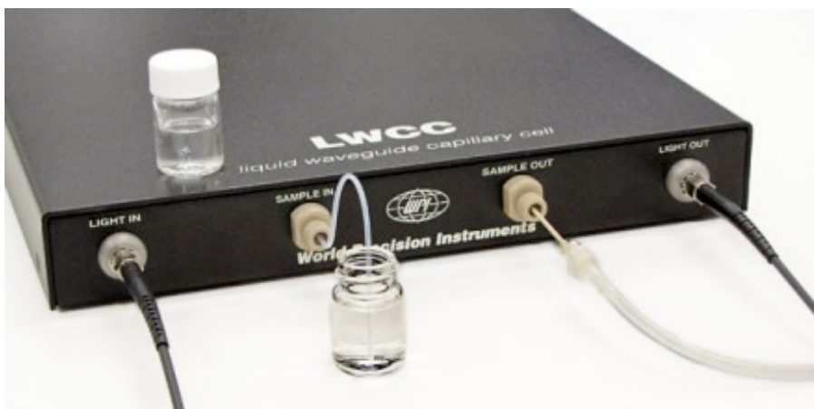
Fig. 1 LWCC system with connections attached
