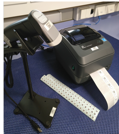
Fig. 2 (left) Medium-sized labels with the possibility of adding sample information in addition to the Data Matrix.
