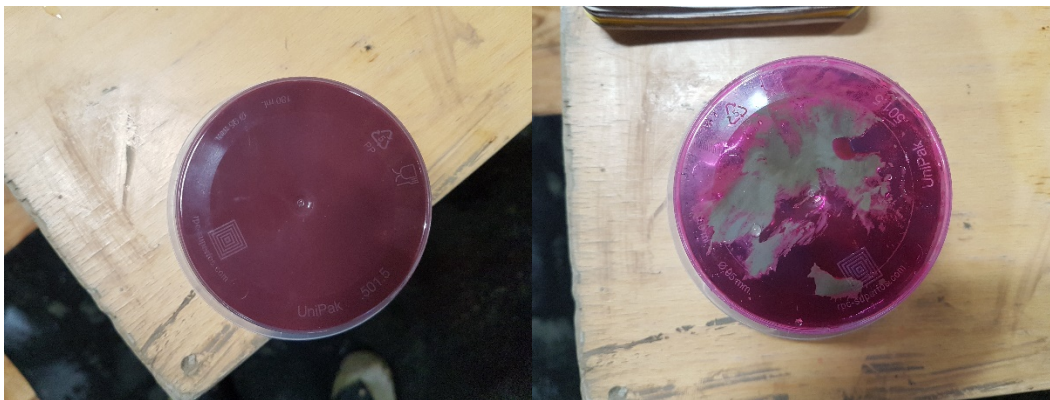
Fig. 2 Well-mixed sample (left) and not sufficiently mixed sample (right).
