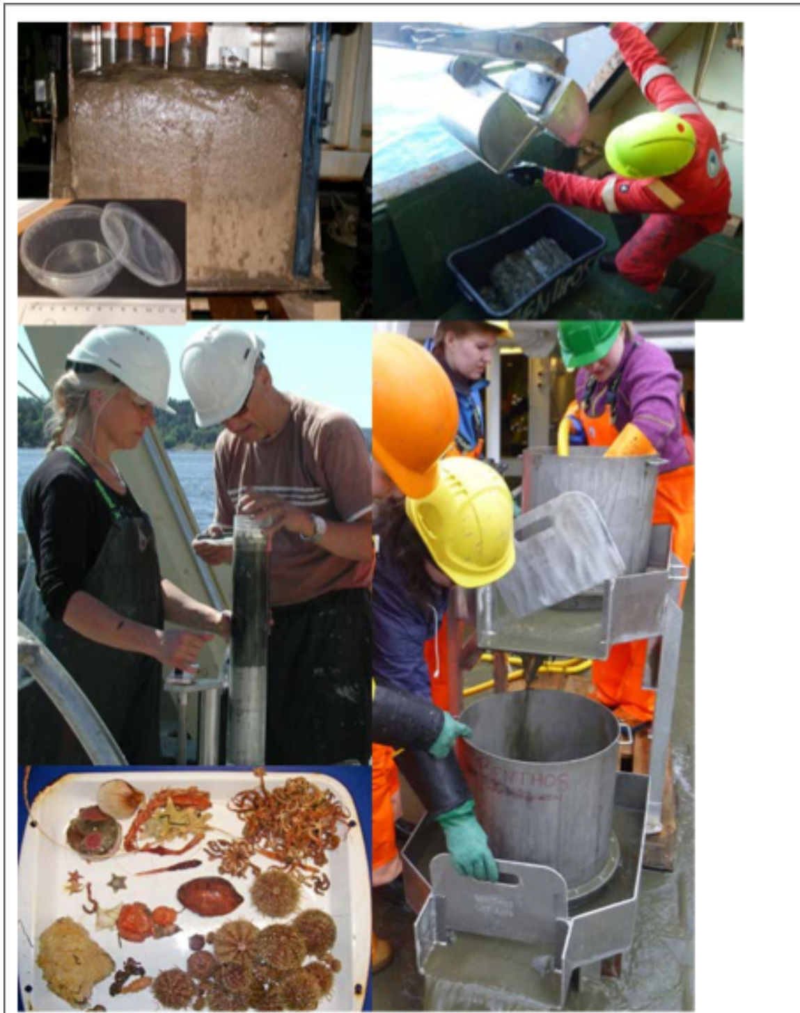
Fig. 2 Biological sample taking procedures. Top left) Box core sampling, top right) emptying van Veen grab into a tub for sieving, middle left) Sectioning Gemini core (and sampling container), bottom left) sorting trawl sample, bottom right) sieving macrofauna (from van Veen / box core). (Photos S. Hess, B. Bluhm).
