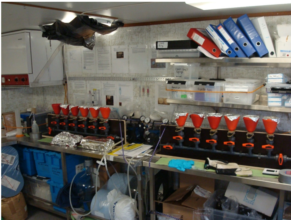
Fig. 1 Example of a filtration set-up.
