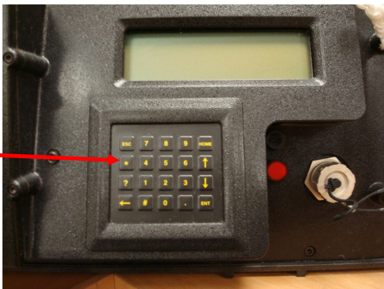
Fig. 7.11.1-1 Display and buttons of the Turner Design AU10 Fluorometer, * button is indicated by the red arrow
