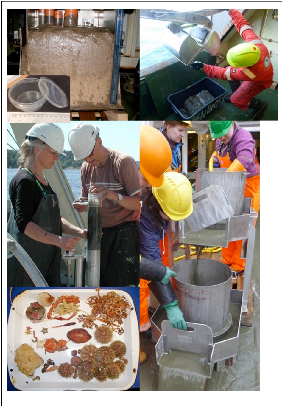
Fig. 10.3-1 Biological sample taking procedures. Top left) Box core sampling, top right) emptying van Veen grab into a tub for sieving, middle left) Sectioning Gemini core (and sampling container), bottom left) sorting trawl sample, bottom right) sieving macrofauna (from van Veen / box core). (Photos S. Hess, B. Bluhm).
