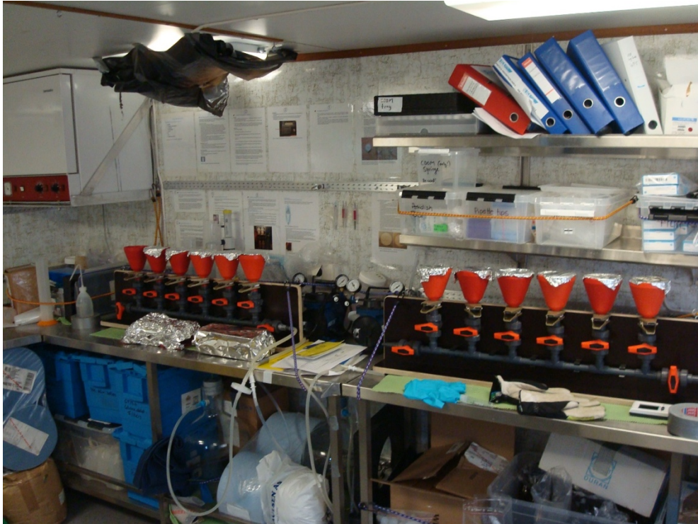
Fig. 7.11-1 Example of a filtration set-up.
