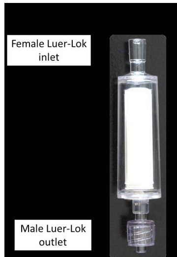
Fig. 7.15-1 Left: Sterivex filter with indication of inlet and outlet; Right: Peristaltic pump filtration set-up
