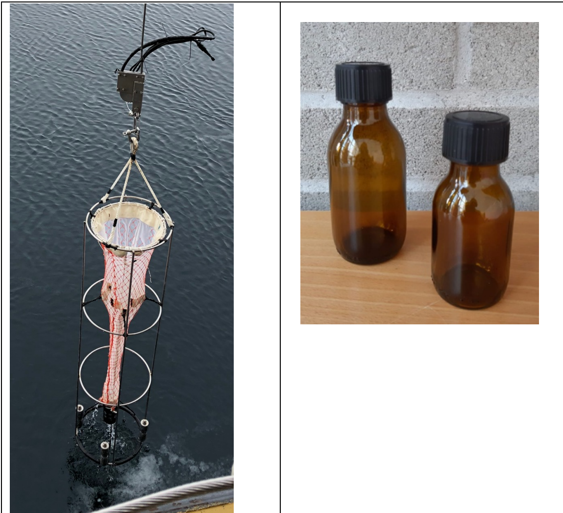
Fig. 9.1-1 Phytoplankton net from IMR net with steel frame (left hand side) and collection of brown glass sampling bottles (right hand side)
