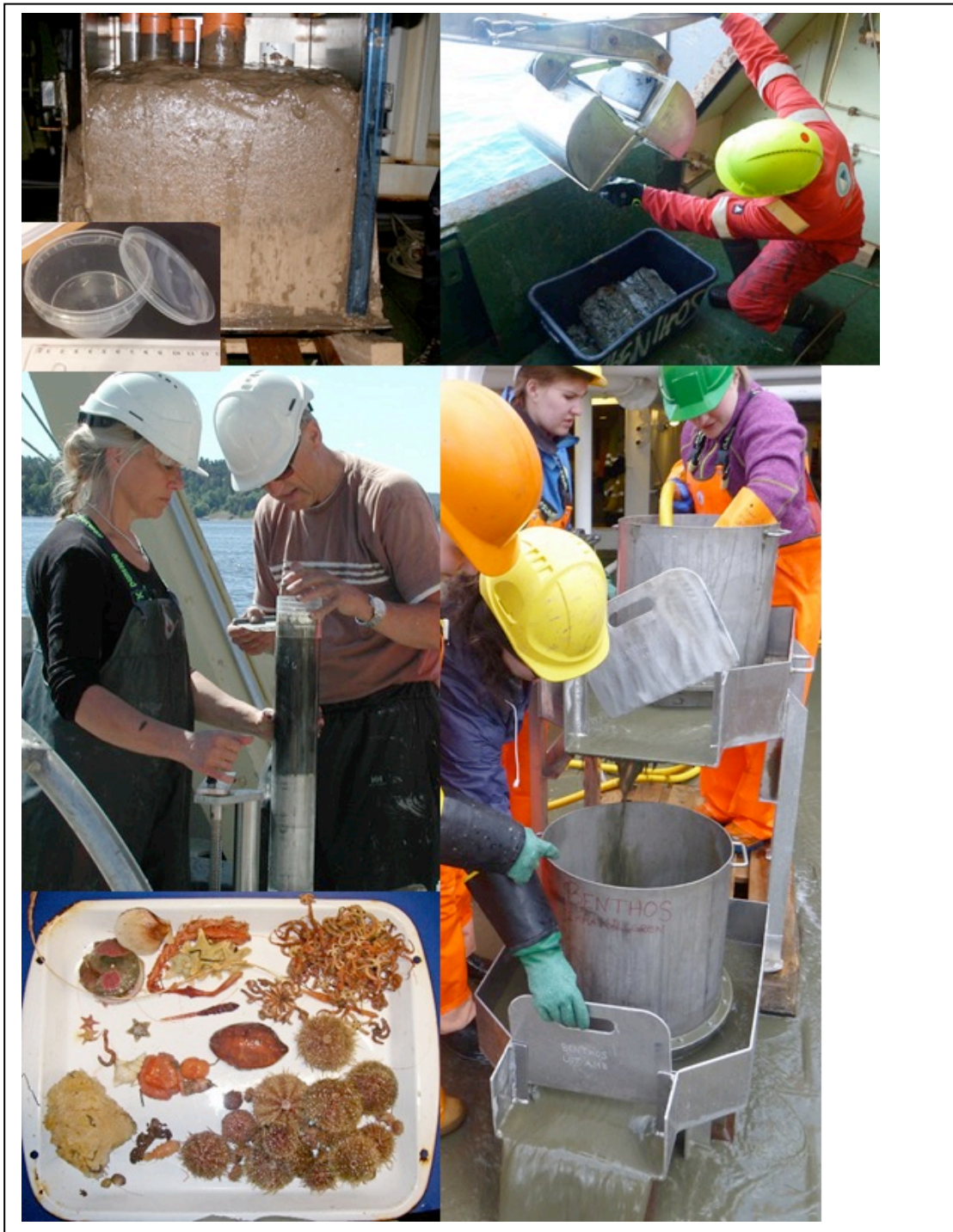
Fig. 10.3-1 Biological sample taking procedures. Top left) Box core sampling, top right) emptying van Veen grab into a tub for sieving, middle left) Sectioning Gemini core (and sampling container), bottom left) sorting trawl sample, bottom right) sieving macrofauna (from van Veen / box core). (Photos S. Hess, B. Bluhm).
