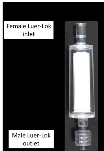
Fig. 7.17-1 Left: Sterivex filter with indication of inlet and outlet; Right: Peristaltic pump filtration set-up
