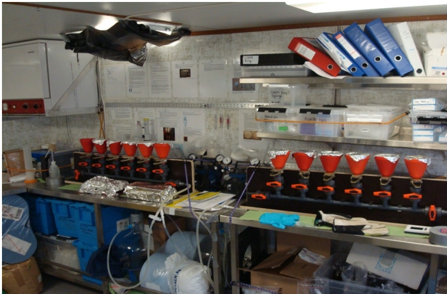
Fig. 7.13-1 Example of a filtration set-up.
