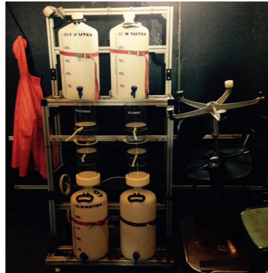
Fig. 7.16-2 Example of filtration tower (AWI-made; contact Uwe John) to concentrate large protists and small mesozooplankton (right side)
