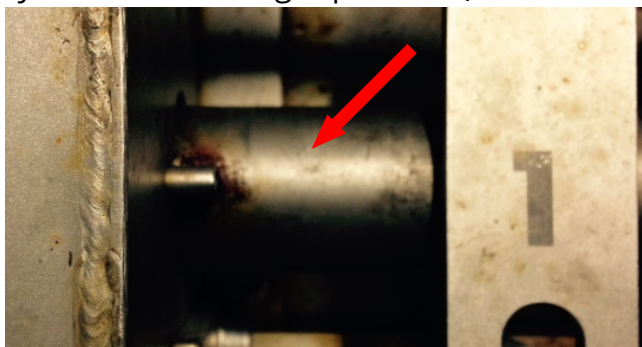
Fig. 9.3.1-1 There is a small pin on the rotating cylinder which should point straight at the pin seen here.
