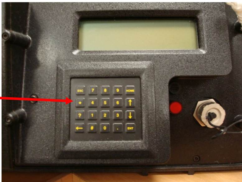
Fig. 7.13.1-1 Display and buttons of the Turner Design AU10 Fluorometer, * button is indicated by the red arrow
