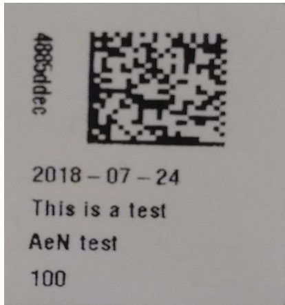
Fig. 2.2-1 (left) Medium-sized labels with the possibility of adding sample information in addition to the Data Matrix.
