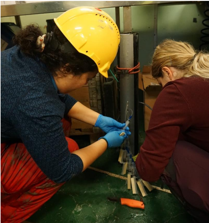
Fig. 10.4.11-1 What it looks like when the rhizons are attached to the syringes causing a vacuum with the wooden stopper.
