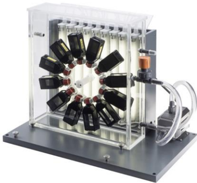
Fig. 7.27-1 Hydrobios ICES incubator (www.hydrobios.de)
