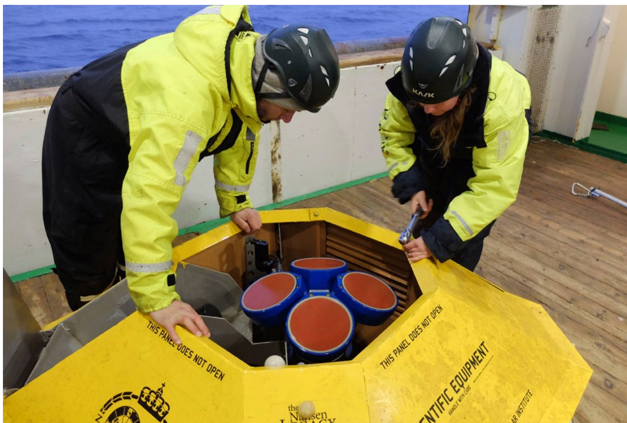
An upward looking ADCP is prepared for deployment. The instrument will sit at the bottom of the Barents Sea and measure the speed and direction of ocean currents.
