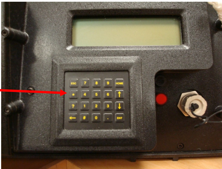
Fig. 7.13.1-1 Display and buttons of the Turner Design AU10 Fluorometer, * button is indicated by the red arrow
