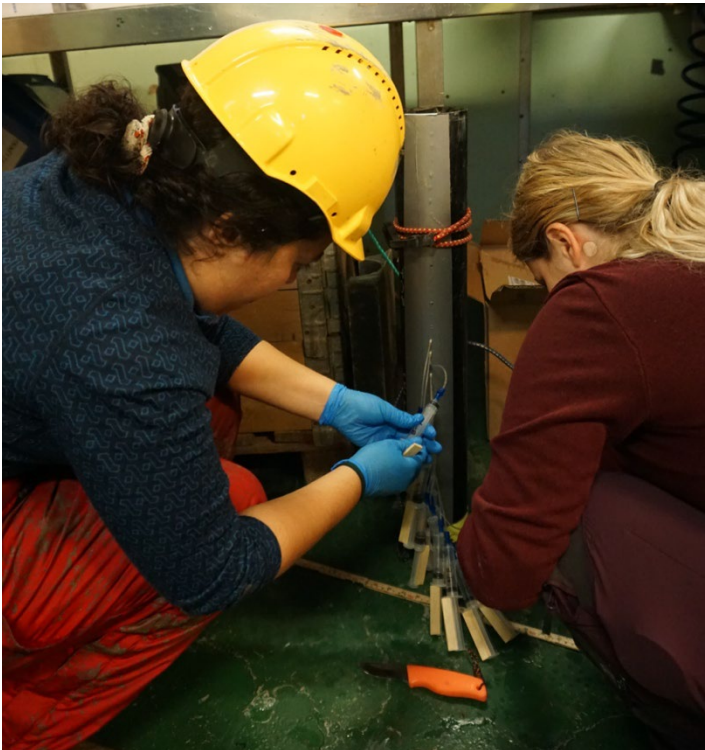
Fig. 10.3.11-1 What it looks like when the rhizons are attached to the syringes causing a vacuum with the wooden stopper.
