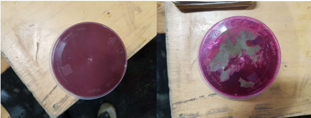
Fig. 15.1.1.1-2: Well-mixed sample (left) and not sufficiently mixed sample (right).
