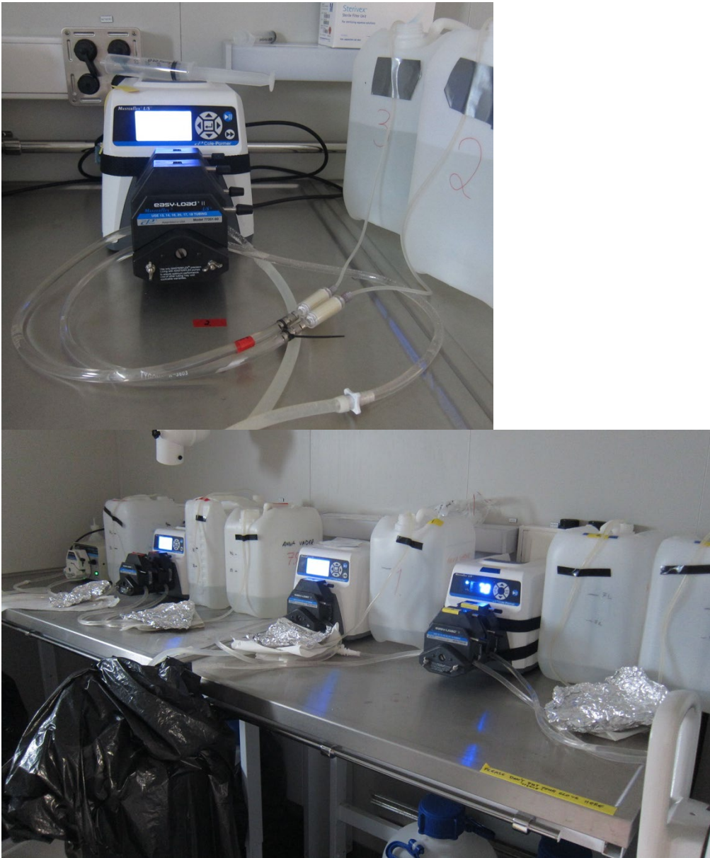
Fig. 7.18-1 Peristaltic pump filtration set-up
