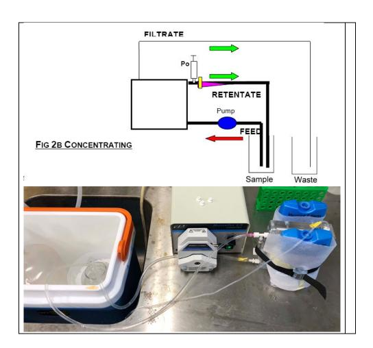
**Fig. 7.14-1** Tangential flow filtration (TFF) concentration of phytoplankton (D. Vaulot: www.protocols.io)
