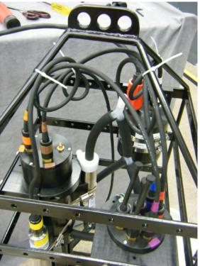
**Figure 6.5.1-1** – Ac-s system. Left: Global view of the system with the ac-s on the left and the DH4 on the right of the picture. Right: Zoom on the upper part of the system.
