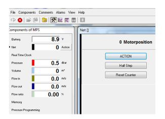
**Fig. 9.4.1-4** Mark Net in the right menu and use Half step to reset rotating cylinder
