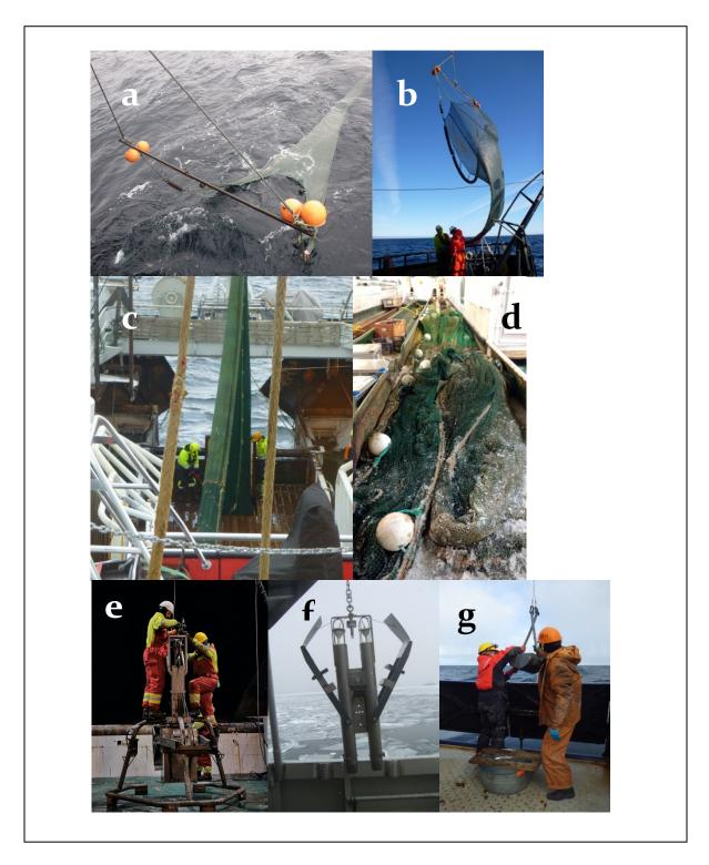
**Fig. 10.2-1** Sediment / benthic sampling gears to be used during Arven etter Nansen cruises. A-B) Beam trawl, C-D) Campelen trawl (photos: B. Bluhm), E) box core (photo: R. Hjertenes), F) Gemini corer (photo S. Hess), G) van Veen Grab. (photo B. Bluhm).
