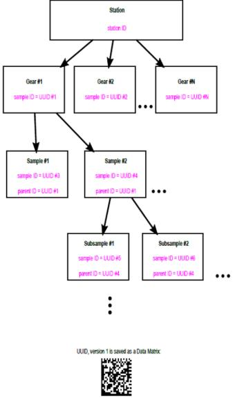
**Fig. 2-1** The hierarchical system with sample/subsample IDs used to trace samples and data within the project.
