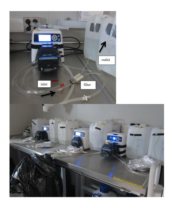
Fig. 7.16-1: Peristaltic pump filtration set-up
