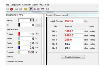
**Fig. 9.4.1-3** Pressure programing. Unlock pressure needs to be deeper than opening depth of Net 1
