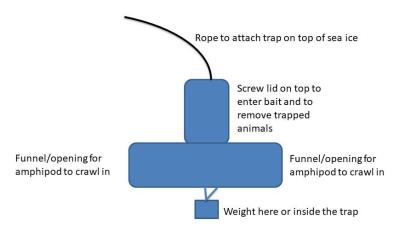
Home-made amphipod traps, cheap and simple
