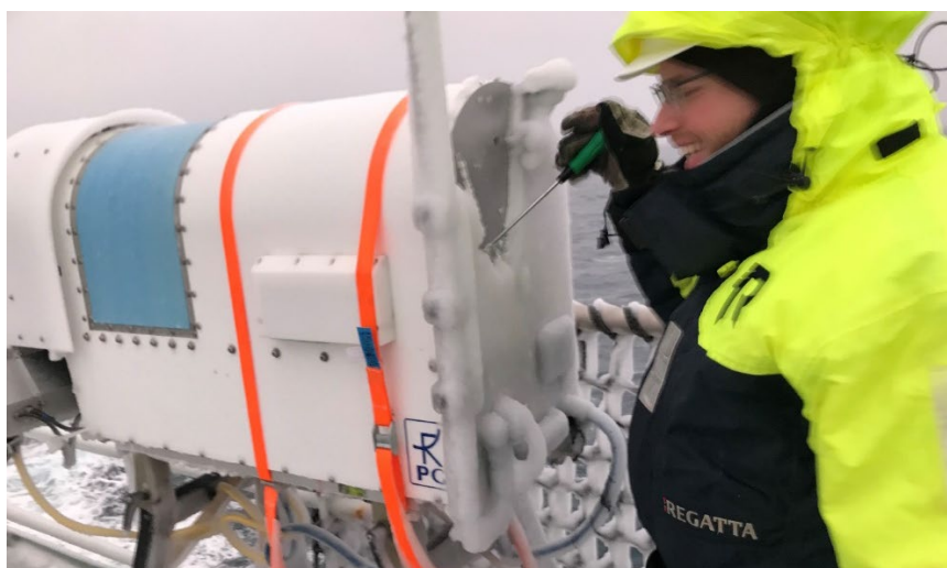
Figure 17: Removal of the ice layer from the HATPRO microwave radiometer.
