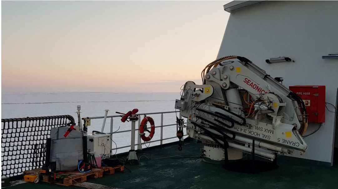
Figure 16: The lidars installed on starboard on the helicopter deck.
