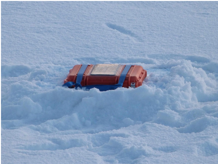
Figure 18 : waves in ice loggers 'v1' are contained in a single Pelican case (total weight around 5kg, dimensions around 30cm x 18cm x 16cm).
