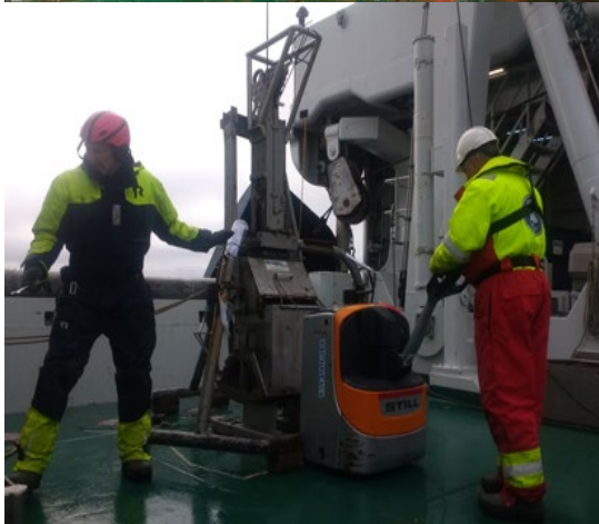
Figure 10. Sampling tools used for benthic sampling during Q3: Top: Campelen 1800 shrimp trawl. Bottom: giant box corer. Photo B. Bluhm.
