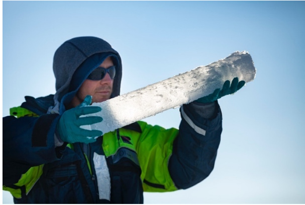
Figure 16. More than 30 sea ice cores were drilled to provide enough material for all the parameters. Photo: Christian Morel (christianmorel.net).
