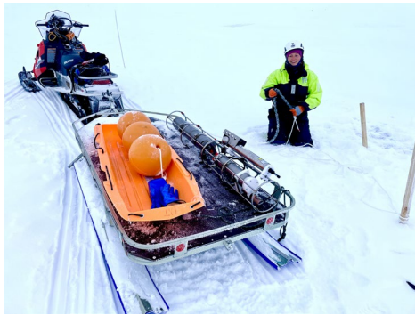
Figure 5-1. The retrieval of the pCO 2 and DO sensors from the lead site on the 13th September (to the right on the sled). Bonnie Raffel was performing the retrieval with Marius Bratrein (also photographer).
