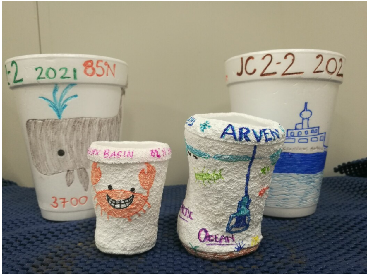
Regular sized foam cups (back) and cups shrunk from being sent to the bottom of the ocean (front). Photo: Arunima Sen, UNIS
