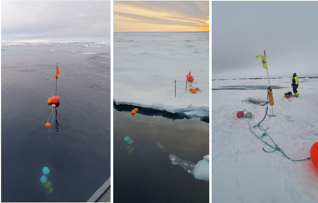
Figure 6-6. Deployed pelagic sediment traps under thin ice conditions found at P7 (a) and off the side an ice floe at P8-P11 (b). In addition, at P8-P11 under-ice and gel sediment traps were deployed through an ice hole (c). Traps were deployed between 28/08/21 and 16/09/21 on the JC2-2 AeN Nansen Legacy cruise. Photos: Jessie Gardner.
