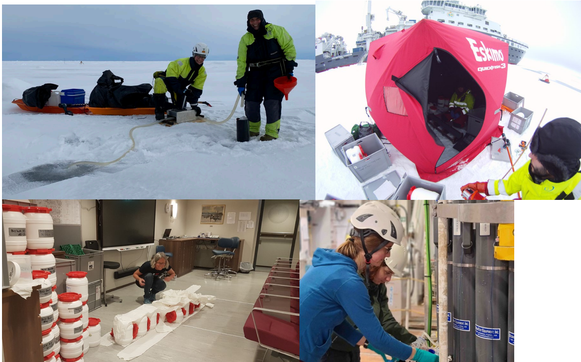
Figure 6-2: Sea ice and water sampling. Top left: Sampling water from a frozen meltpond using auger and a handpump. Photo: Anna Vader. Top right: Coring and sectioning of light sensitive ice-cores for sampling of biological parameters. Photo: Even Sletteng Garvang. Bottom left: Drying of containers for ice-core sections under “clean” conditions in the Kronprins Haakon auditorium. Photo: Miriam Marquardt. Bottom right: Water sampling from niskin bottles. Photo: Bodil Bluhm
