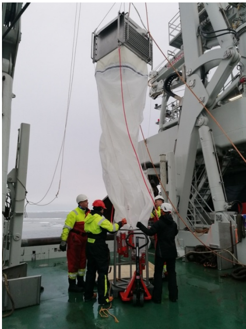
Figure 6-1 Multinet mammoth, sampling capacity 9 depths and area of opening 1 m 2 . Photo: Christine Gawinski.
