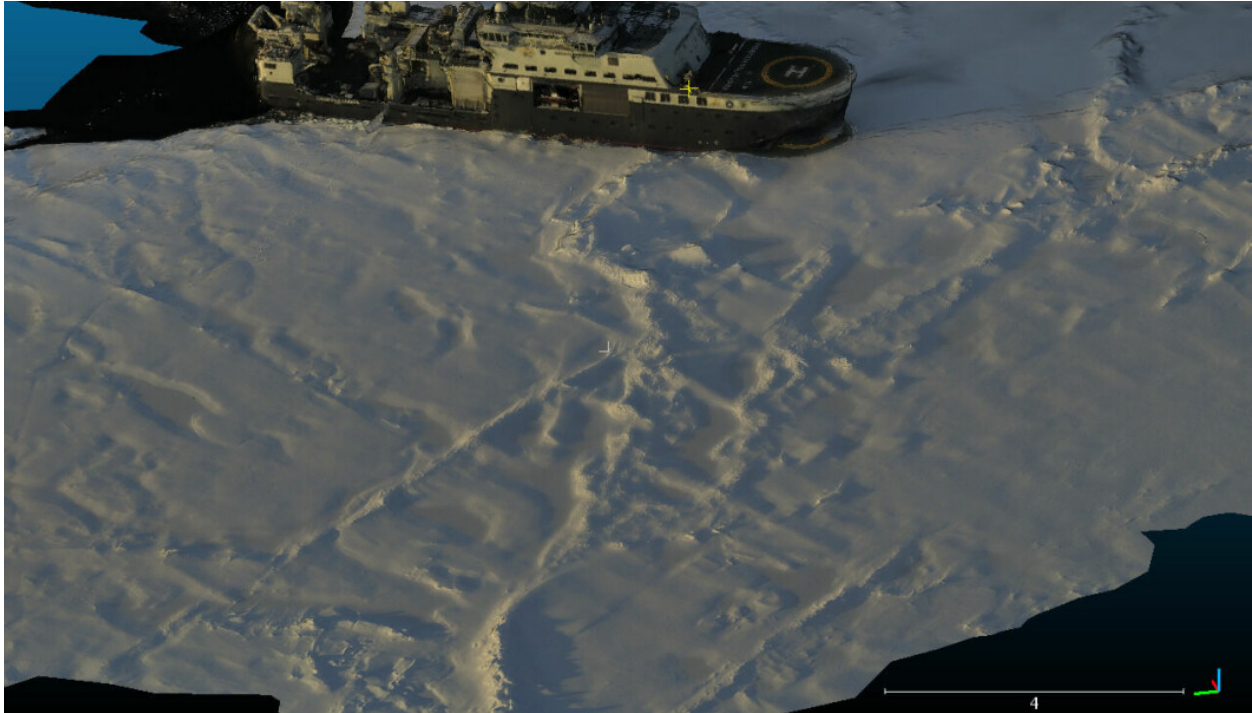
3D model of sea ice and FF Kronprins Haakon, generated from drone imagery Photo: Adam Steer, NPI
