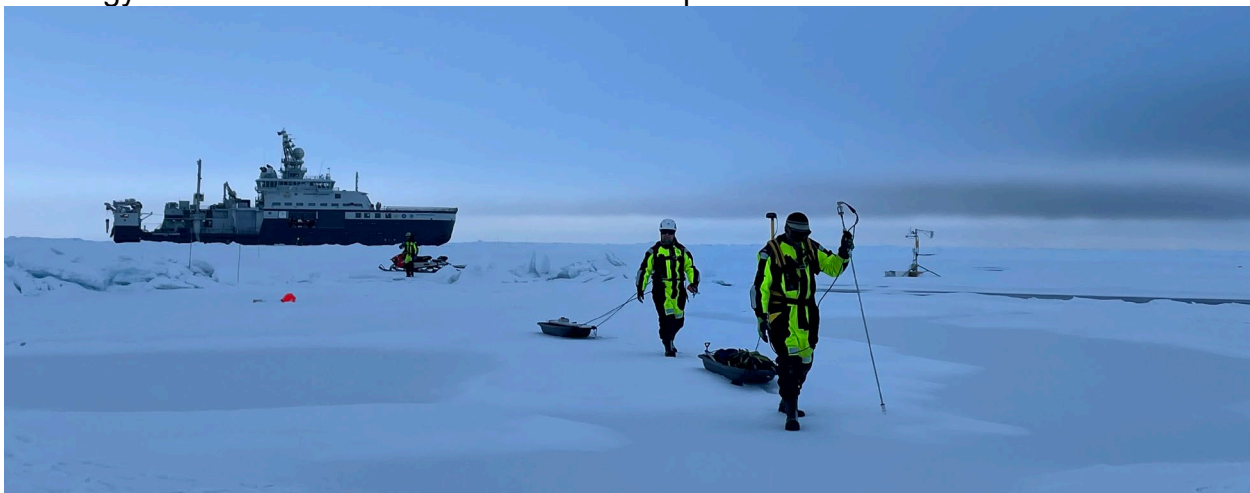
Figure 4-9 Snow and ice thickness soundings using a Magnaprobe and Geophex GEM-2 instrument, respectively. Photo: C. Lockwood-Ireland.
