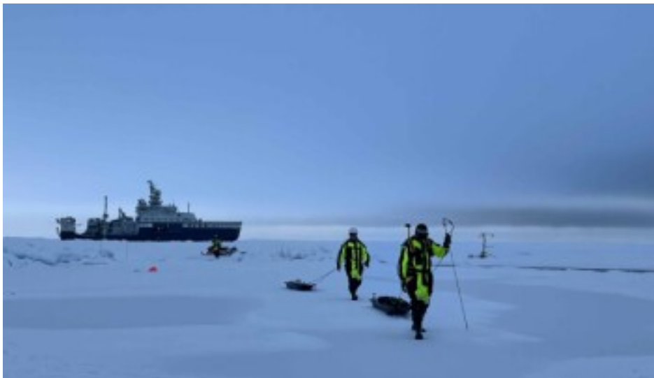
Adam Steer and Anca Cristea measuring snow depth with an automated probe, and ice thickness with a sled towed electromagnetic sounding ski. Photo: Christine Lockwood-Ireland
