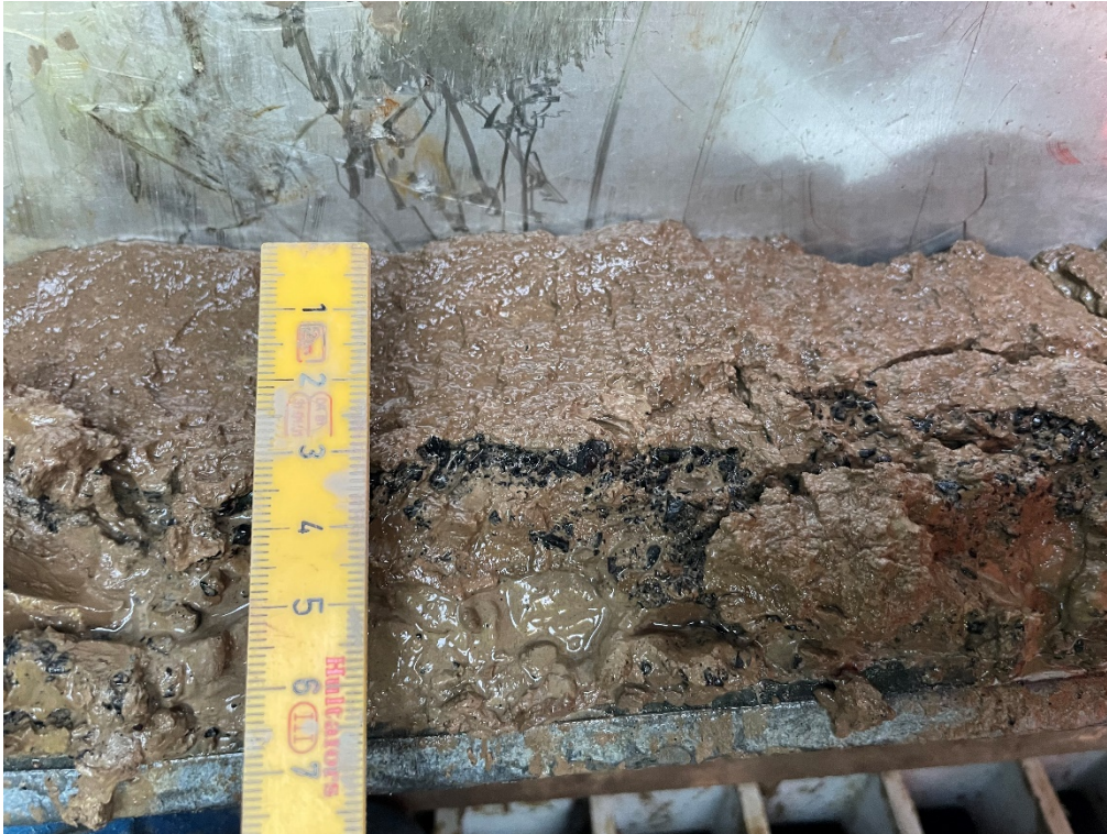
Figure 6-13 Prominent layer of black clasts observed on the outside of the box core 1 at P10.
