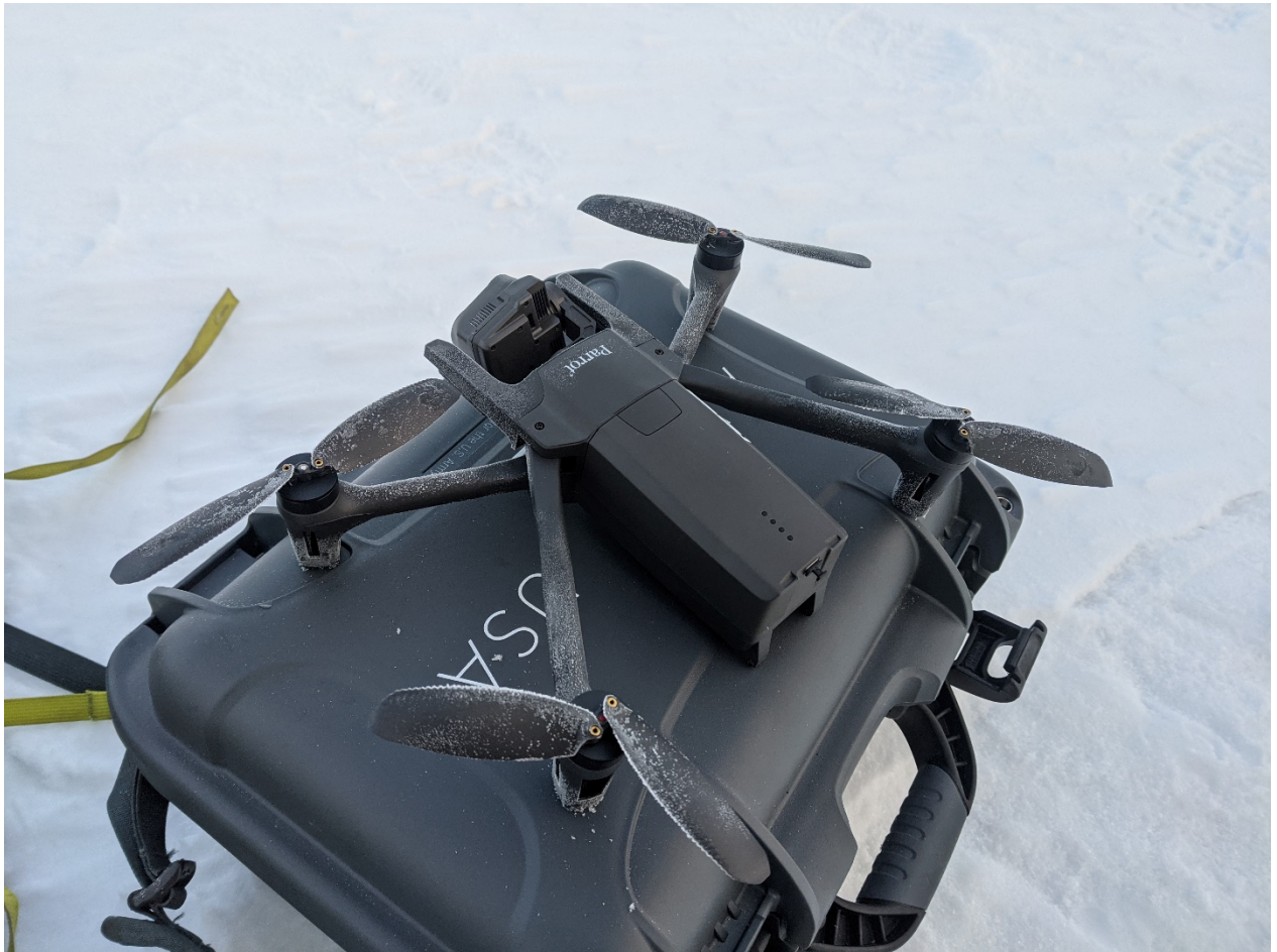
Figure 9: Icing after drone operations at P7, in -17 C air temperatures
