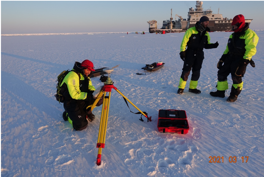
Figure 10: Adam Steer (NPI) is setting up Leica GPS base station at P7. Photo: Dmitry Divine (NPI).
