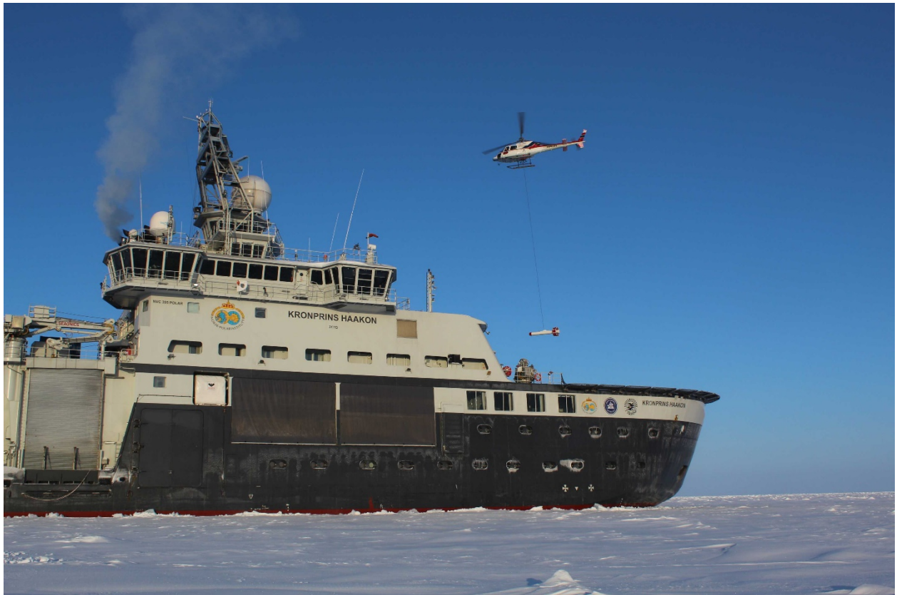
Helicopter take-off with the 'EM bird' ice thickness sensor hanging below, and the stereo camera system (Photo: Sebastian Gerland, Norwegian Polar Institute).
