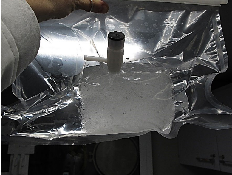
A section of an ice core in a vacuum packed bag ready for melting to analyse for carbonate chemistry and inorganic nutrients (Photo: Libby Jones, Institute of Marine Research).
