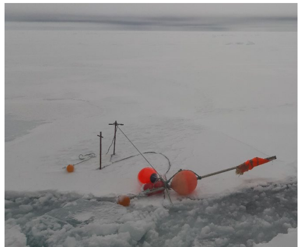
Figure 14: Deployed sediment trap under ice conditions (left) and on an ice floe (right) during SSQ3 in August 2019
