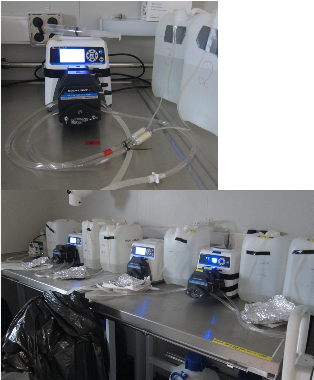
Fig. 7.17-1 Peristaltic pump filtration set-up
