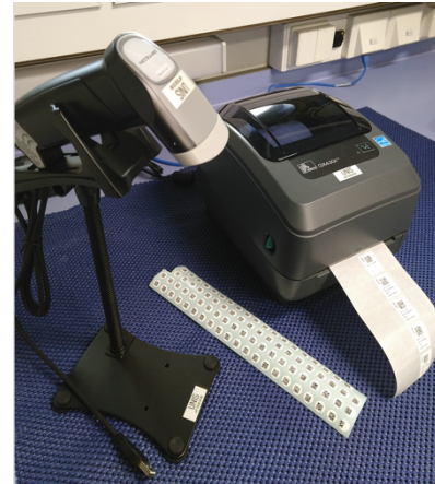
Fig. 2.2-1 (left) Medium-sized labels with the possibility of adding sample information in addition to the Data Matrix.
