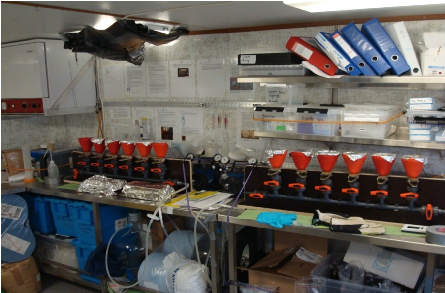
Fig. 7.13 - 1 Example of a filtration set-up.
