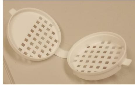
Fig. 7.10-1 Plastic capsule to be used for flash freezing of 25mm particle absorption filters
