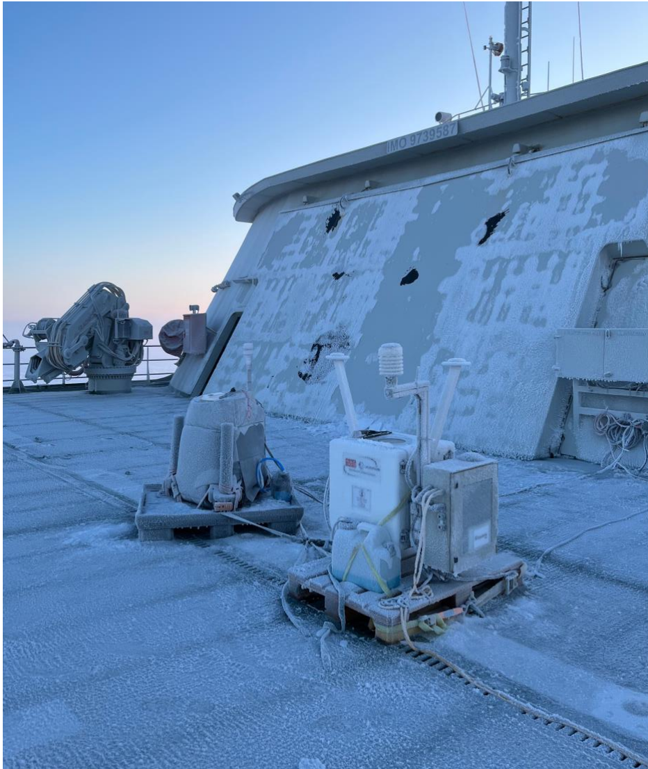
Figure 2: Lidars location and setup on the Helicopter Deck.
