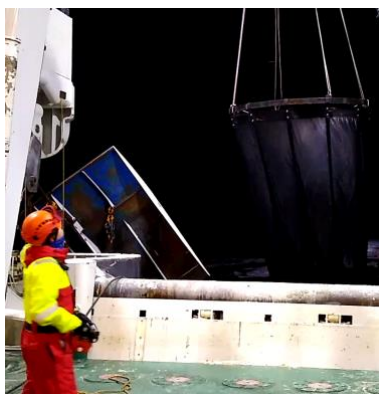
Figure 11. Deployment of the MIK net (midwater ring-trawl) at the A-frame of RV Kronprins Haakon.
