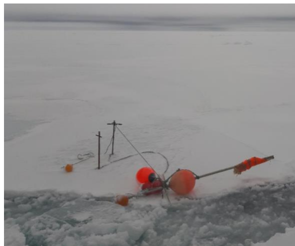
Figure 21. Deployed sediment trap under ice conditions (left) and on an ice floe (right) during SSQ3 in August 2019.
