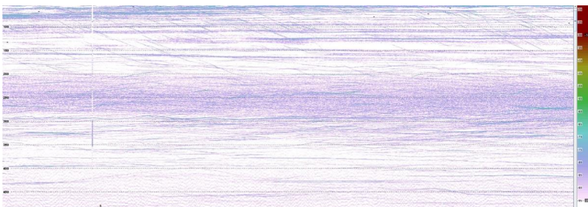
Figure 8. Example echogram from the ship based echosounder for the P7 station. The echogram show the 70kHz echosounder. The vertical range is depth from surface to 500 m. The horizontal axis is time.
