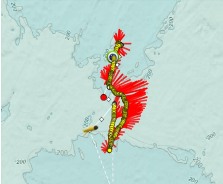
Figure 7: Odin's track as displayed on the Slocum Fleet Mission Control dashboard, showing the surface fixes (yellow circles) and the depth-averaged currents (red sticks). The deployment was on the northern end of the transect. Odin completed one southward transect across the front, turned northward and it was recovered as it approached the front once more.
