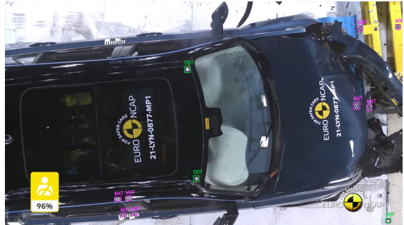
Figure 5: Sample output from the developed pipeline. This image shows the small size of the target regions. The different marker types are found accurately in the high resolution image.
