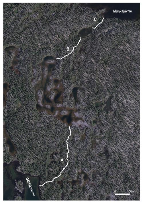
Figure 4. The three parts of the fence between Lake Muŋkajávrre and Gáldaksavon (a part of the Pite River). Two unnamed lakes form part of the fence. Since the direction changes at almost every joint, the fence winds through the forest. There were three openings where no log remains could be found, two in part A (5.6 m and 3.2 m wide) and one in part B (6.4 m wide). © Lantmäteriet.
