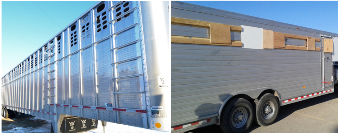
Figure 1. Livestock trailer used to transport caribou from British Columbia to Ontario (16.15 meter Wilson Trailer model PSAGL-400 on left) and Alaska (7.32 meter gooseneck trailer on right) in April 2017. Trailers were modified to reduce light but maintain ventilation and equipped with video cameras to remotely monitor caribou in real-time during transport.
