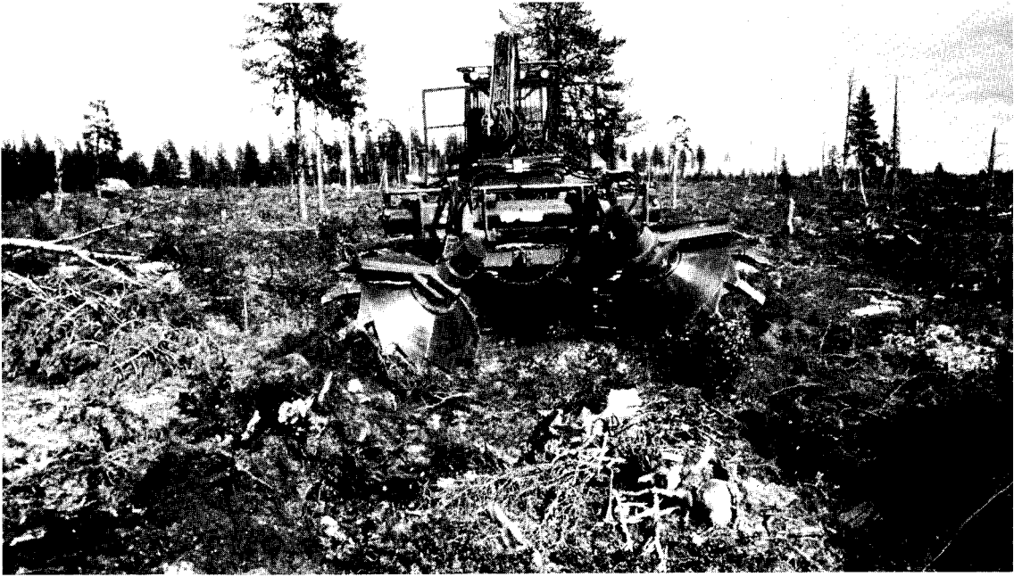
Photo 1 a,b. The main site preparation methods to be used are harrowing and ploughing. A) deep cultivator (=plough), B) scarifier of harrow type. (Photo: O.E.)
